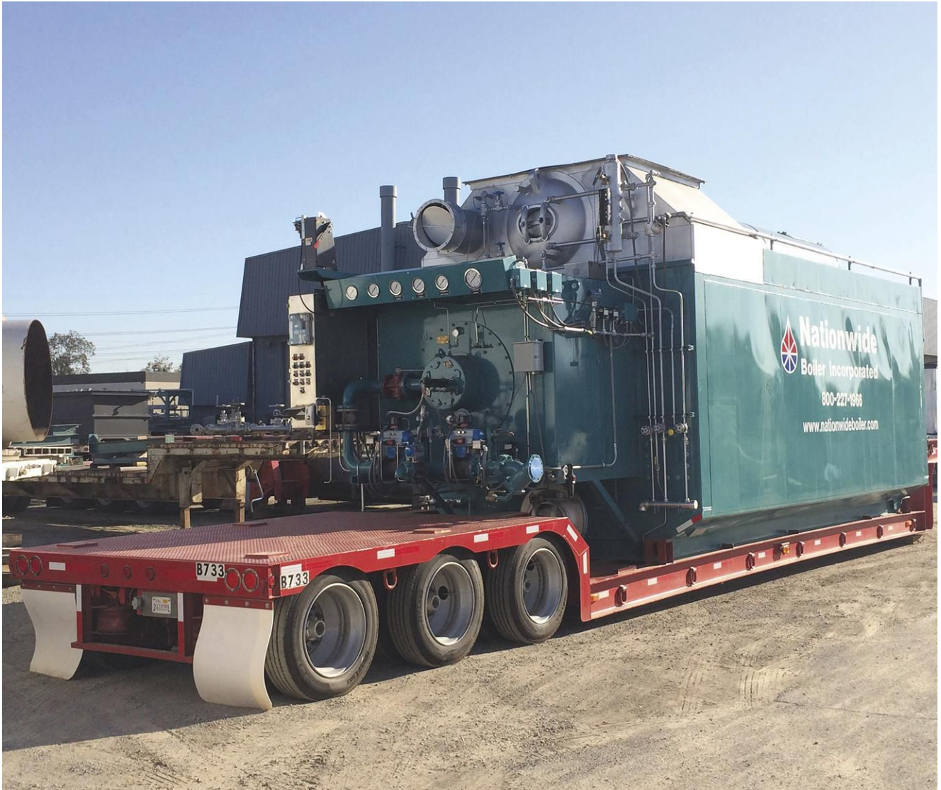
This is the same 82,500 lb/hr boiler after a full reconditioning. The boiler was inspected and tested, and any necessary repairs and replacements were made.
