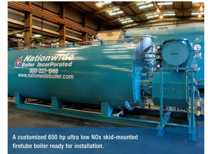
A customized 650 hp ultra low NOx skid-mounted firetube boiler ready for installation.
