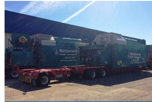
Trailer-mounted boilers can be dispatched on short notice and require no special cranes or rigging at either the storage yard or the user's facility.
