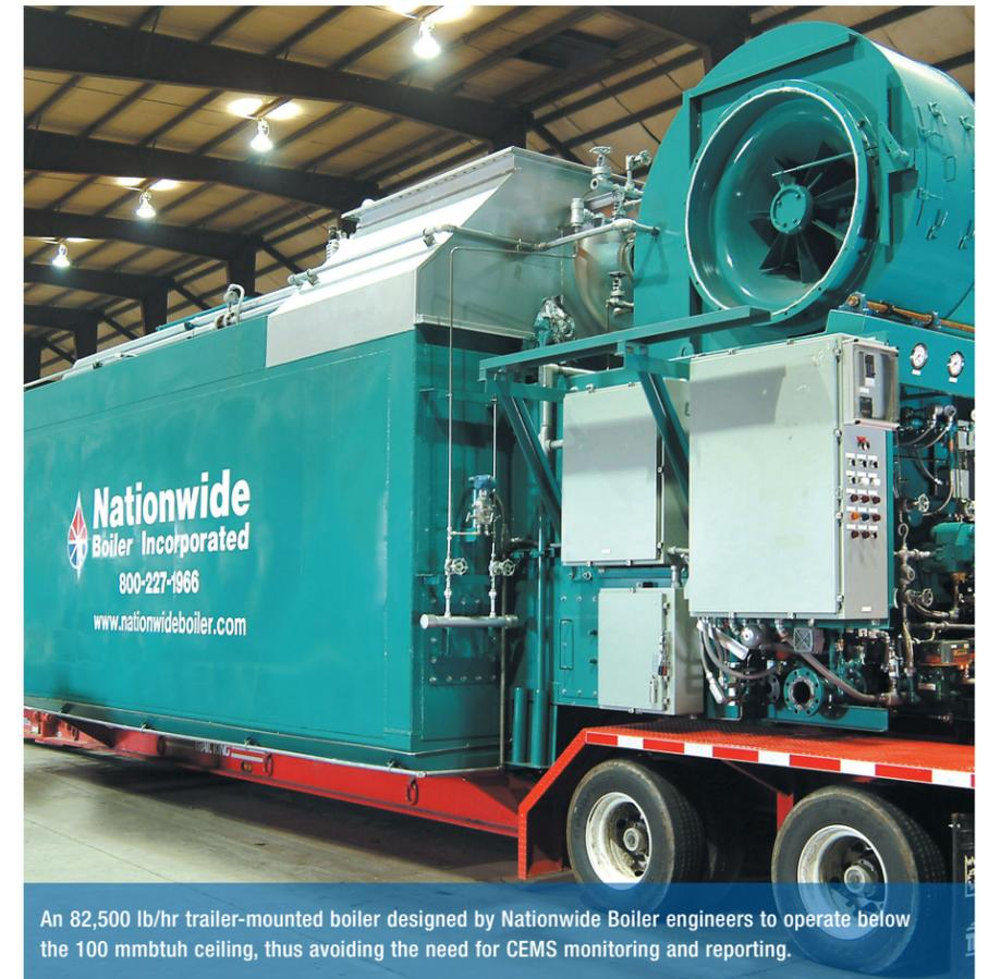
An 82,500 lb/hr trailer-mounted boiler designed by Nationwide Boiler engineers to operate below the 100 mmbtuh ceiling, thus avoiding the need for CEMS monitoring and reporting.
