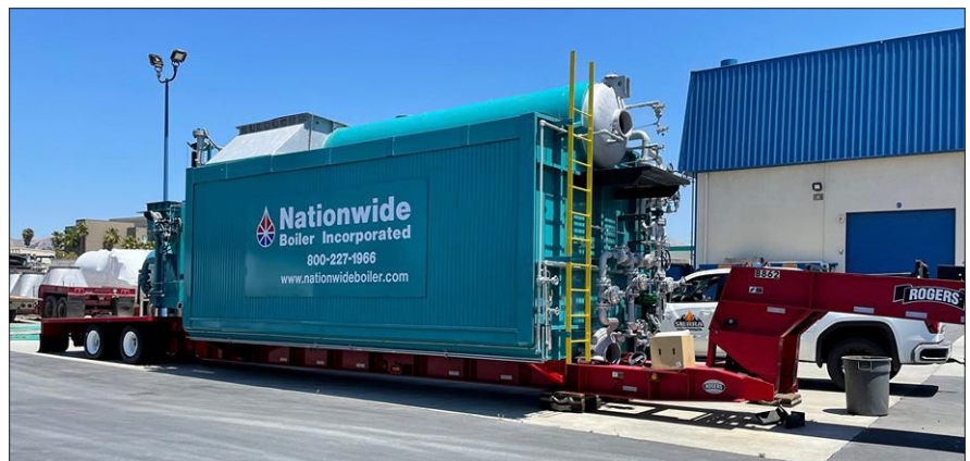
FIGURE 2. One of Nationwide's 100,000-pound-per-hour, 399-psig, trailer-mounted rental boilers. The company now has six of these units in its rental fleet.
