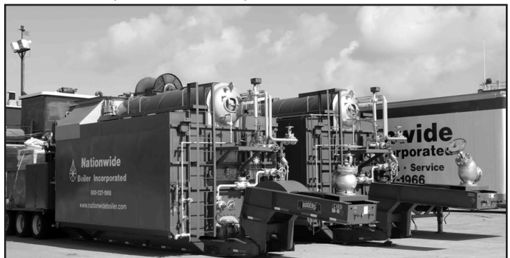
Two 70,000 lb/hr trailer-mounted Nebraska package boilers and a feedwater van waiting to be loaded on to the Mignon.
